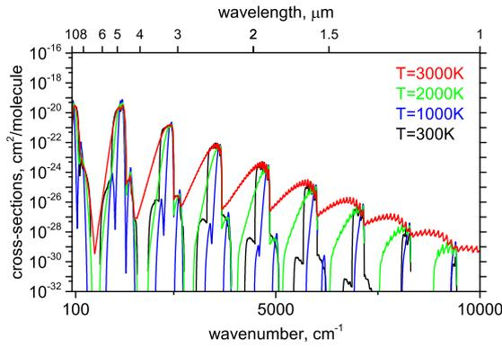
**Figure 10.** PO absorption spectrum at  $T = 300$  (bottom), 1000, 2000 and 3000 (top) K, presented with cross-sections on a logarithmic scale. A Gaussian profile with a Half Width at Half Maximum (HWHM) =  $10 \text{ cm}^{-1}$  was used.
