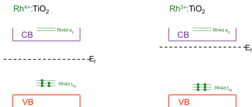
Figure 39: Schematic band diagram showing the change in Fermi level energy between Rh (III) and Rh (IV) doped TiO 2
