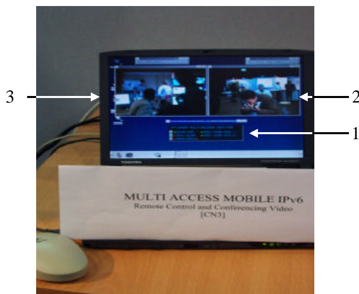
Figure 18: The Ericsson Multi-Access control screen in Tübingen - transmitted via MIPv6 (1), local low-rate video transmitted to Tübingen (2), low-rate video transmitted from Tübingen (3) - all transmissions via MIPv6 in Ericsson’s Multi-Access implementation
