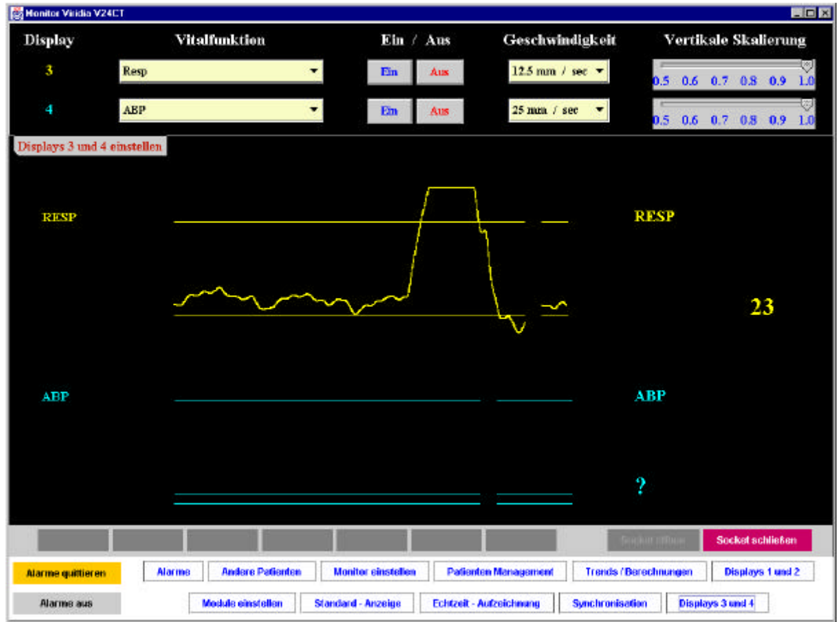
Figure 39 : The configuration for the vital parameters of the two lower displays
