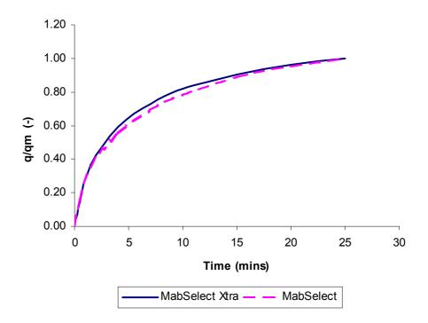
Fig 2.17 – Normalised version of the uptake kinetic curves for MabSelect and MabSelect Xtra using higher concentration of hlgG (3mg/ml) and an impeller speed of 145rpm. The uptake rate shows to be very similar for the two media.
