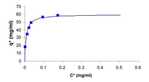
Fig 2.6 – Adsorption Equilibrium – Prosep Ultra. Experimental data for Prosep Ultra fitted using Langmuir isotherm and the maximum capacity and dissociation constant were determined using the Solver function in Excel
