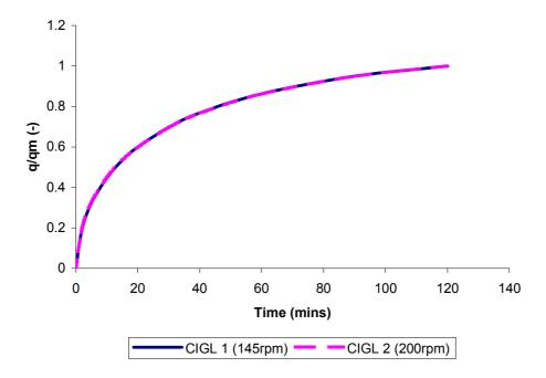
Fig 2.13 - Uptake kinetic curves for two samples of CIGL where maximum capacity at the end of adsorption for each sample equals to 1. The two graphs showed to be reproducible.
