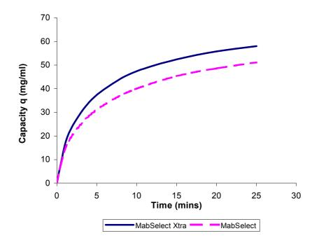
Fig 2.16 – Uptake kinetic curves for MabSelect and MabSelect Xtra using higher concentration of hIgG (3mg/ml) and an impeller speed of 145rpm. The uptake rate shows to be very similar for the two media.
