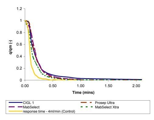
Fig 2.19 – Desorption kinetic curves for MabSelect, MabSelect Xtra, Prosep Ultra and CIGL. Impeller speed of 145 rpm was used except for Prosep Ultra where 200rpm was used. Desorption rate shows to be very similar for all four media.
