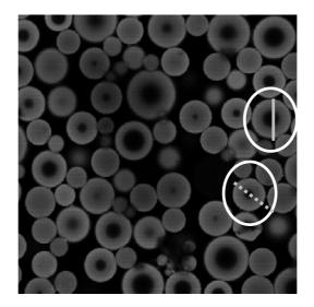
Fig 3.3 - Image of beads seen under the microscope at 30 mins. The images of the chosen beads are from the centre and of different sizes ( $50\mu$ m and  $70\mu$ m). The line across the bead helps produce the intensity profile across that section as seen in figure 3.4
