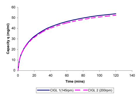
Fig 2.12 - Uptake kinetic curves for two samples of CIGL where the impeller speed of 145rpm and 200rpm was used to check mixing characterisation and reproducibility.
