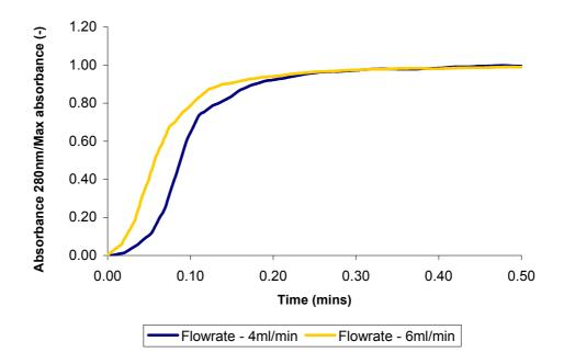
Fig 2.11 – Response time here is defined as the amount of time before the system stabilises and shows a constant UV 280nm reading. This equilibration time (response time) is recorded at 4ml/min and 6ml/min flow rate which shows to be ~20-25sec.
