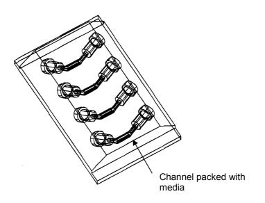
Fig 3.1- Flow cell with a channel of diameter 0.1cm and a length of 1cm was used to pack  $\sim 8\mu$ l of media, which could be placed under an inverted confocal microscope.
