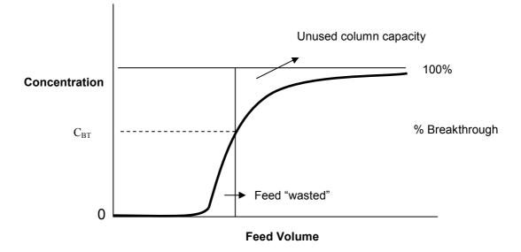
Fig 1.9 – Breakthrough curve
