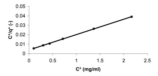
Fig 2.7 – Hanes Plot – CIGL. Linearised form of Langmuir isotherm for CIGL. 1/slope gives the maximum capacity and y intercept equals to  $Kd/Q_{max}$ . The equation for the line is y=0.0163x + 0.0039 with an R<sup>2</sup> value of 0.9997. Here  $Q_{max}$  = 61.5 and Kd = 0.024mg/ml
