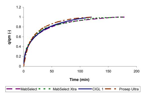
Fig 2.15 – Uptake kinetic curves for MabSelect, MabSelect Xtra, Prosep Ultra and CIGL where maximum capacity at the end of adsorption for each media equals to 1. The uptake rate shows to be very similar for all four media.
