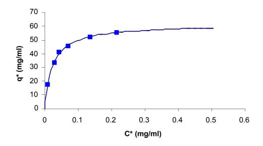
Fig 2.8 – Adsorption Equilibrium – CIGL. Experimental data for CIGL fitted using Langmuir isotherm and the maximum capacity and dissociation constant were determined using the Solver function in Excel
