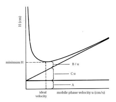
Fig 1.7 – A typical Van Deemter Plot (Deemter et al., 1956)
