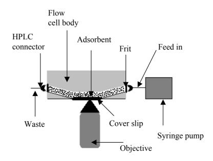
Fig 3.2 - Flow cell setting under confocal microscope. 2mg/ml hlgG was passed through the channel at 0.1ml/min flowrate with a syringe pump.
