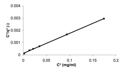
Fig 2.5 – Hanes Plot – Prosep Ultra. Linearised form of Langmuir isotherm for Prosep Ultra. 1/slope gives the maximum capacity and y intercept equals to Kd/Q<sub>max</sub>. The equation for the line is y=0.01630x + 0.00013 with an R<sup>2</sup> value of 0.99927. Here Q<sub>max =</sub> 61.3 and Kd = 0.008mg/ml
