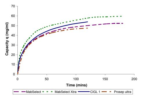
Fig 2.14 – Uptake kinetic curves for MabSelect, MabSelect Xtra, Prosep Ultra and CIGL. Impeller speed of 145 rpm was used except for Prosep Ultra where 200rpm was used. Maximum capacity determined at 120 mins.
