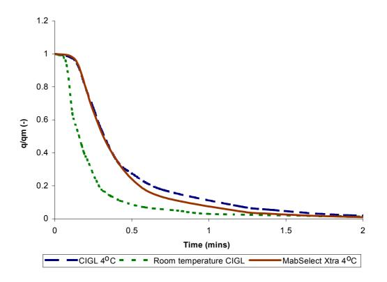
Fig 2.20 – Desorption carried out on CIGL and MabSelect Xtra at 4°C to slow down the rate of desorption. Similar results showed for the two media at 4°C. Impeller speed of 145 rpm was used
