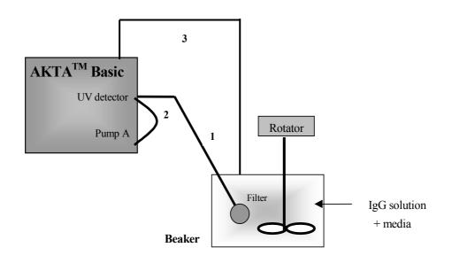
Tube 1 – Connected from filter to outlet of UV detector Tube 2 – Connected from inlet of UV detector to Pump A of  $AKTA^{TM}$  Basic. Tube 3 – Waste loop
