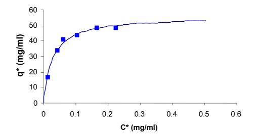
Fig 2.2 – Adsorption Equilibrium – MabSelect. Experimental data for MabSelect fitted using Langmuir isotherm and the maximum capacity and dissociation constant were determined using the Solver function in Excel.
