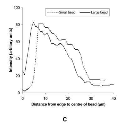
Fig 3.4 - Intensity profile across a small bead ( $\sim$ 50µm) and a large bead ( $\sim$ 70µm) at A; 10mins, B; 20mins and C; 30 mins time intervals. The distance travelled by hIgG to the centre of the bead with time can be estimated from the profile
