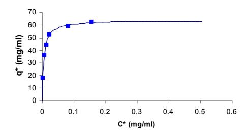
Fig 2.4 – Adsorption Equilibrium – MabSelect Xtra. Experimental data for MabSelect Xtra fitted using Langmuir isotherm and the maximum capacity and dissociation constant were determined using the Solver function in Excel
