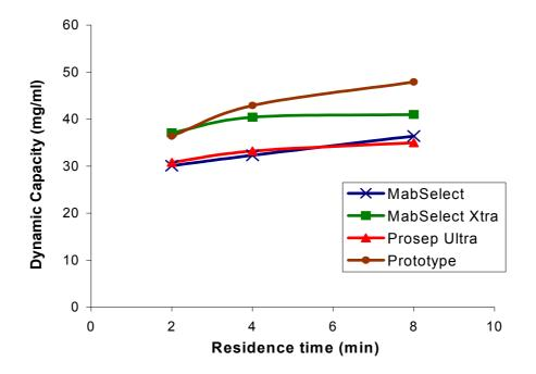
Fig 2.9 – Dynamic capacity determined at 2min, 4min and 8min residence time for MabSelect, MabSelect Xtra, Prosep Ultra and CIGL. 0.66cm Omnifit column with a bed height of 6cm was used. Loading was stopped at 20% breakthrough.
