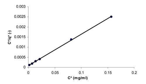
Fig 2.3 – Hanes Plot – MabSelect Xtra. Linearised form of Langmuir isotherm for Mabselect Xtra. 1/slope gives the maximum capacity and y intercept equals to Kd/ $Q_{max}$ . The equation for the line is y=0.01554x + 0.00009 with an R<sup>2</sup> value of 0.99975. Here  $Q_{max}$  = 64.4 and Kd = 0.006mg/ml
