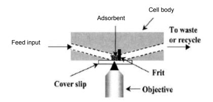
Fig 1.10 – Flow cell set up used to view labelled individual beads under a confocal microscope
