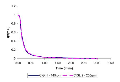
Fig 2.18 – Desorption kinetic curves for two samples of CIGL where the impeller speed of 145rpm and 200rpm was used to check mixing characterisation and reproducibility
