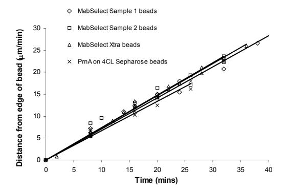
Fig 3.6 - Adsorption rate for different size beads for two different samples of MabSelect, 1 sample of MabSelect Xtra and Protein A immobilised on 4CL Sepharose
