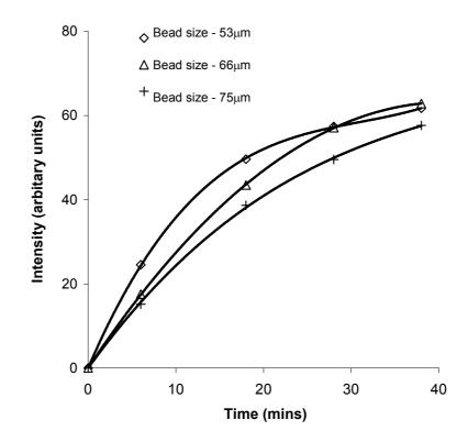
Fig 3.7 - Uptake curves for different size beads of MabSelect Xtra plotted from data calculated from intensity profiles
