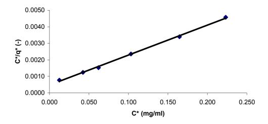
Fig 2.1 – Hanes Plot – MabSelect. Linearised form of Langmuir isotherm for Mabselect. 1/slope gives the maximum capacity and y intercept equals to Kd/Q<sub>max</sub>. The equation for the line is y=0.01813x + 0.00047 with an R<sup>2</sup> value of 0.99832. Here Q<sub>max =</sub> 55.1 and Kd = 0.026mg/ml
