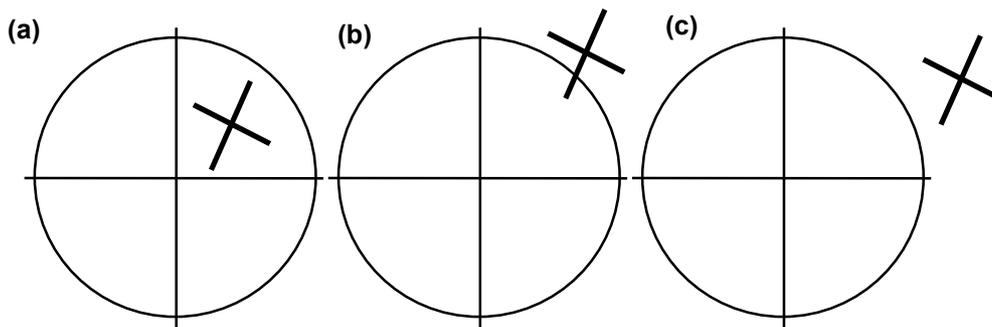
**Figure 3.6** Three possible intersection cases between (circular) region of interest and conic section's semi-axes (After Wood, 1998). (a) Two axes intersect with region - pit, peak or pass, (b) one axis intersects with region - channel or ridge and (c) no intersection - planar.
