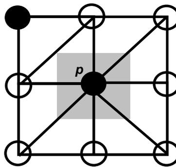
**Figure 3.2** Point  $p$  in a grid (analytical view) and its 7 adjacent neighbours (hollow circles).
