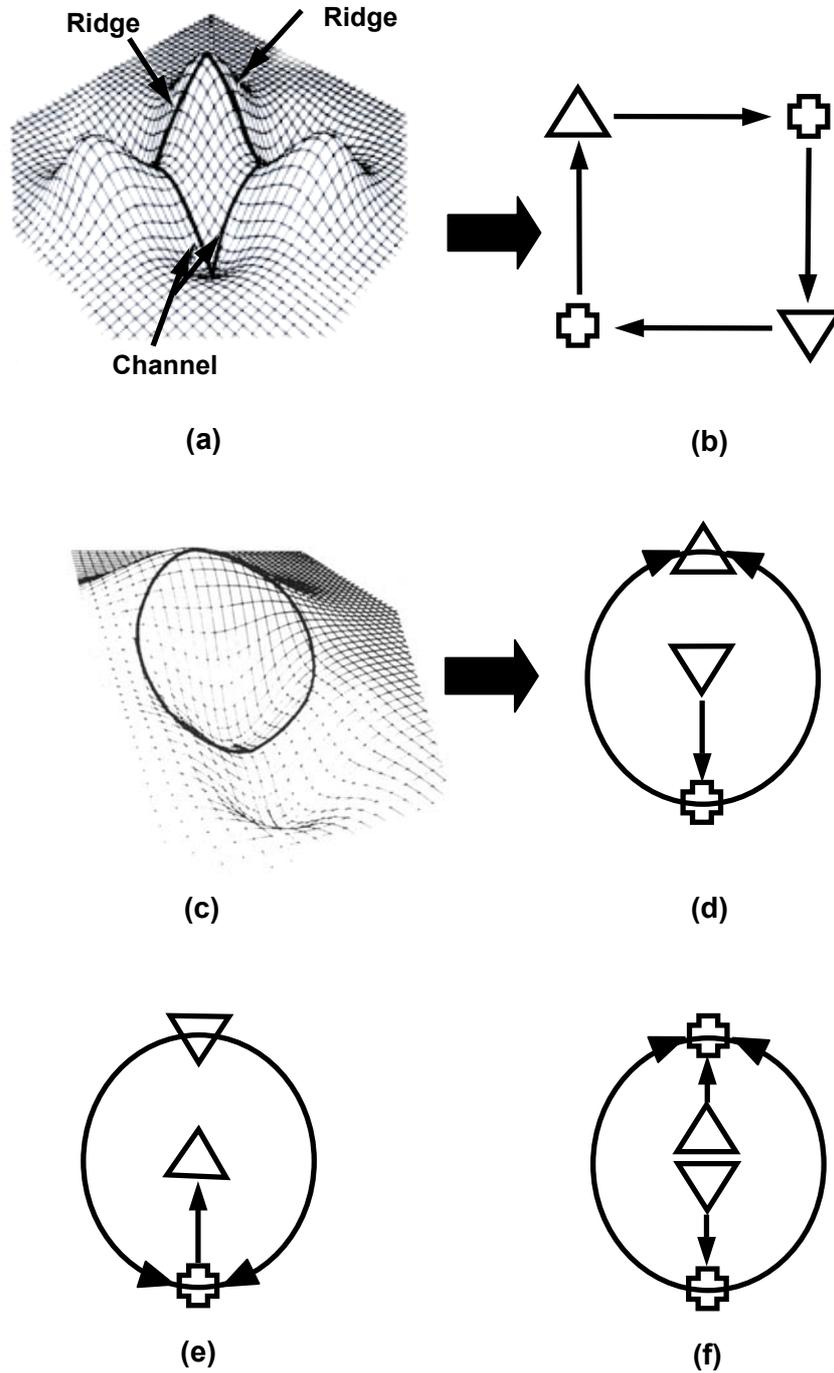
**Figure 2.4** Two examples of slope districts - (a) and (c) and their Critical Point Configuration Graph - (b) and (d) respectively. (e) and (f) are the two other basic types of CPCG.
