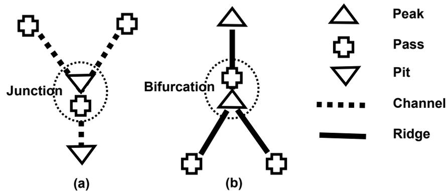
**Figure 2.3** (a) Channel junction and (b) Ridge bifurcation.
