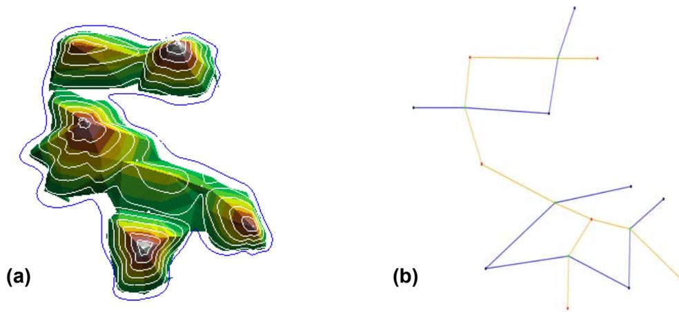
**Figure 4.3** (a) Hypothetical topographic surface and its (b) surface network. Blue contour represents the surrounding pit.
