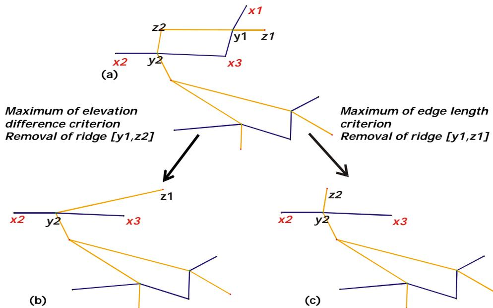
**Figure 4.6** Comparison of the effectiveness for selection of points in the surface network (a) between maximum of elevation difference criterion (b) and maximum of edge length criterion and (c) Note that criterion (b) selects a long ridge due to its low drop in elevation (350).
