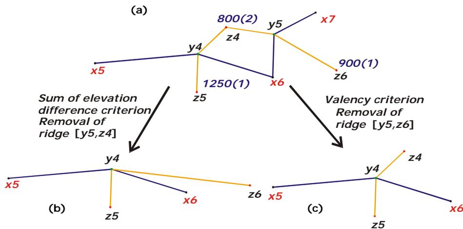
**Figure 4.7** Comparison of the effectiveness for selection of points in a (a) surface network, between (b) sum of elevation difference criterion and (c) valency criterion, showing how criterion (b) can mislead about the ridge/channel crossings. Numbers at peaks in (a) are sum of elevation differences and their valencies (in parentheses).
