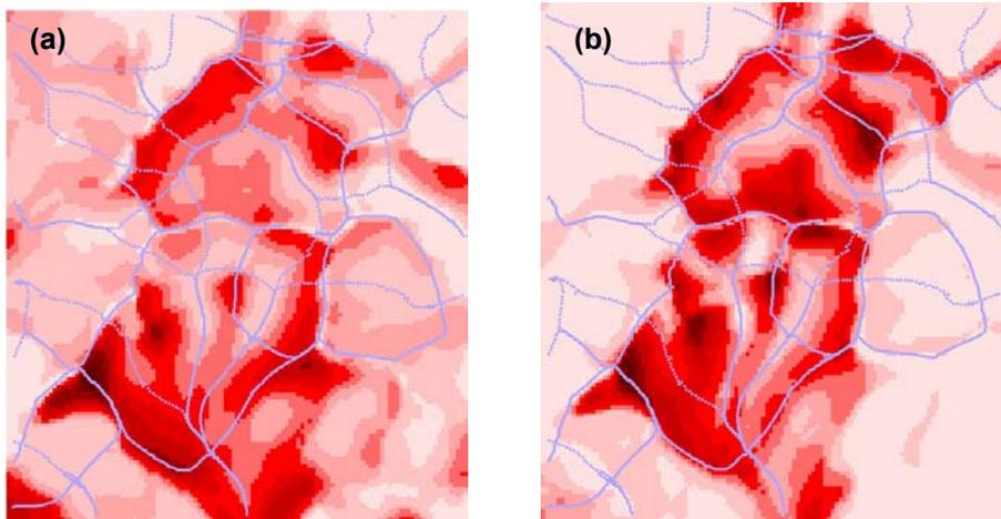
**Figure 5.3** Intervisibility calculations in a part of Isle of Man, based on (a) each grid point (16335 points) and (b) critical points and lines (3975 points). Lighter to darker colour indicates increasing number of observers. The blue line is the surface network.
