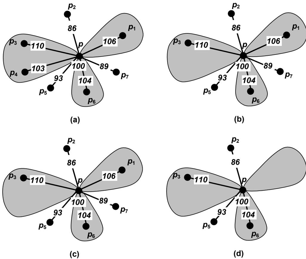
**Figure 3.3** Decomposition of a degenerate pass (Modified from Takahashi et. al, 1995). Figure shows the neighbours and their heights. Higher neighbours are placed inside a grey region. (a) The original neighbour list, (b) the reduced neighbour list, (c) the list in the first turn of the loop in the algorithm, and (d) the final set of neighbours which will define the pass.
