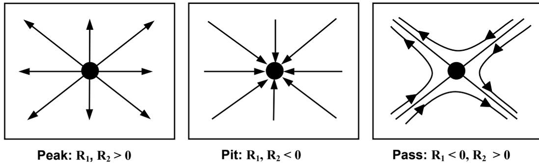
**Figure 3.4** Critical points of the surface and the configuration of their eigenvalues and eigenvectors.  $R_1$  and  $R_2$  are the real parts of the eigenvalues.
