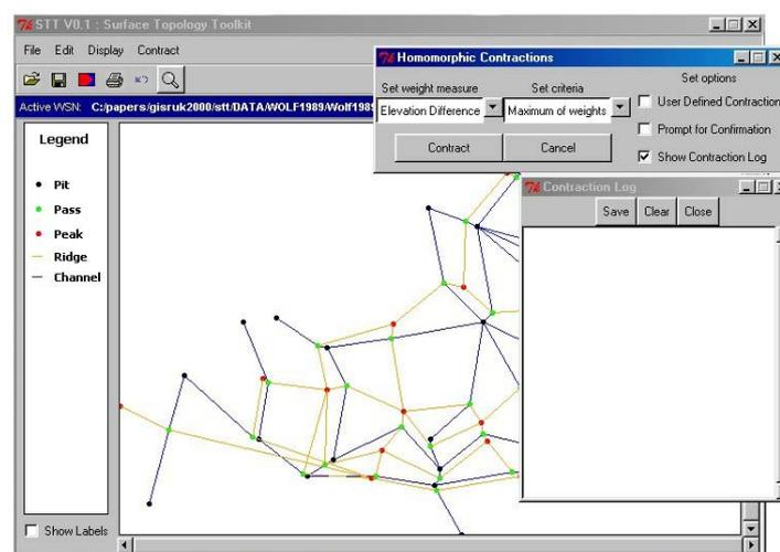
**Figure 4.5** Graphical User Interface of the Surface Topology Toolkit application with the controls for the contractions.
