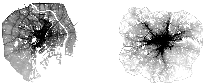
Figures 3 and 4 showing least angle integration (normalised closeness) for metropolitan Tokyo (left) and London within the M25 (right) in each case showing a variant of the 'deformed wheel' structure, with multiple rims in the case of Tokyo
