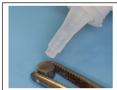
Figure 93: Cyanoacrylate attached to sandblasted Ti-6Al4V rod.
