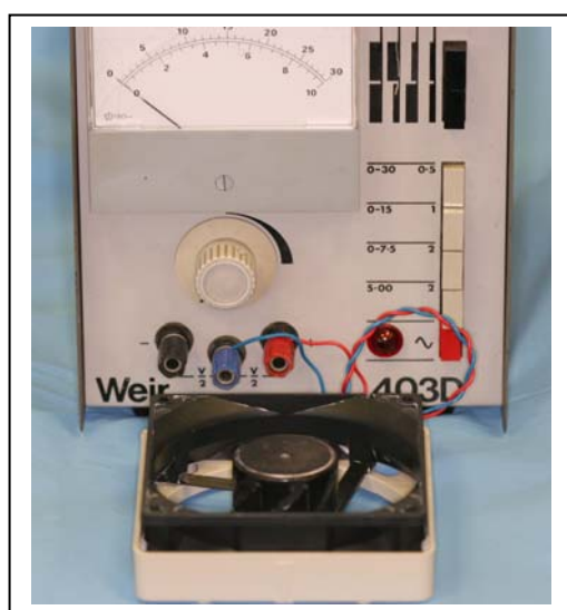
Figure 73: Fan motor wired to Weir 403D power supply.
