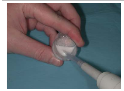
Figure 89: 0.5ml of sol-gel being drawn up in syringe
