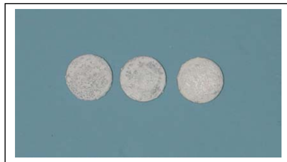
Figure 92: Coated titanium disks after firing
