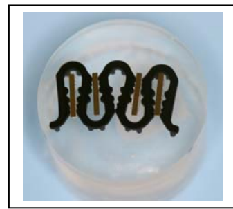
Figure 76: Picture of coated disks after sectioning.
