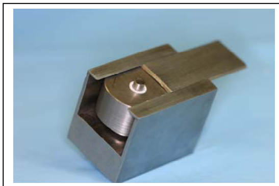
Figure 96: Constructed assembly ready for shear testing.
