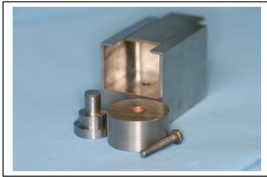
Figure 95: Assembly for mounting disk in Instron Universal load testing machine.
