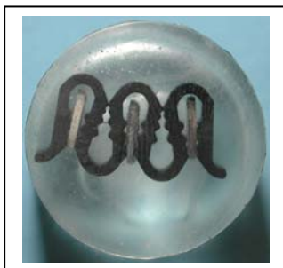
Figure 74: Coated Ti disks mounted in epoxy resin.
