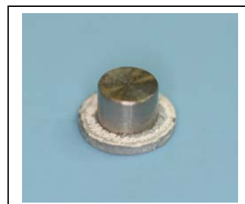
Figure 94: Ti-6Al4V rod attached to coated Ti disk.
