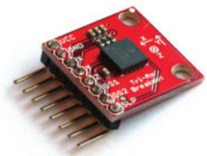
values undergo analog to digital conversion (ADC) and are returned as an integer between 0 and 1023. For the purposes of this project, the accelerometer was configured to read  $\pm 1.5g$  of acceleration and baseline self-assessment and damping values were scripted via the Arduino program in order to constrain the sensor data to useful levels.
