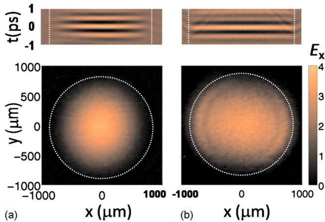
FIG. 3. (Color online) (a) Bottom panel: spatial electric field ( $E_x$ ) distribution at  $t=0$  measured at the output of the waveguide using the terahertz near-field probe; top panel: the corresponding space-time map showing the pulse waveform along the horizontal axis. (b) Similar measurements on a waveguide with the same dimensions however without the dielectric layer.
