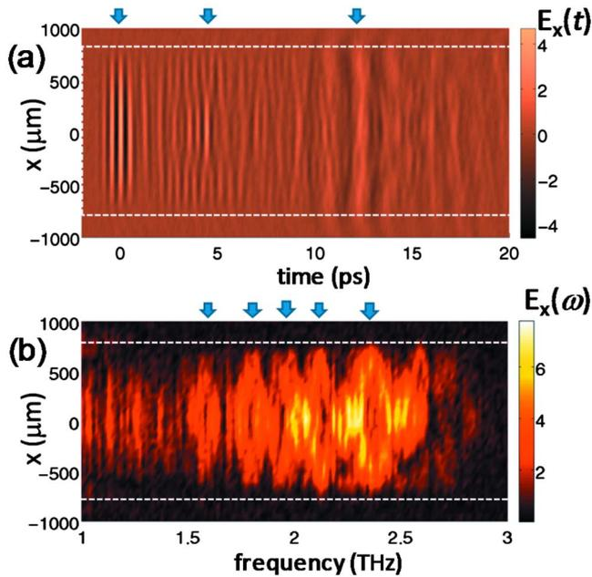
FIG. 1. (Color online) Space-time (a) and space-frequency (b) maps of the horizontal electric field component at the waveguide output measured with the terahertz near-field probe along the horizontal axis. The dashed lines show the inner waveguide wall.
