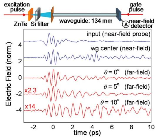
FIG. 4. (Color online) Terahertz pulse waveforms measured in the near-field and the far-field regions. Near-field waveforms are detected by the near-field probe. Angle-resolved waveforms are detected by a photoconductive antenna in the far-field zone. The top waveform shows the input pulse measured by the near-field probe. The schematic diagram shows details of the experimental setup.
