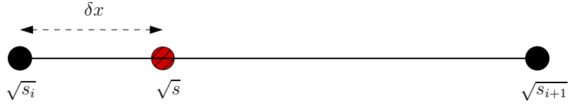
Figure 6.4: Linear interpolation in-between grid points
