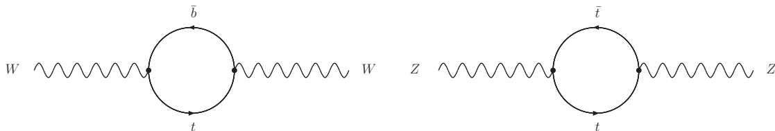
Figure 2.3: One-loop radiative corrections to the W and Z boson masses due to the top quark.
