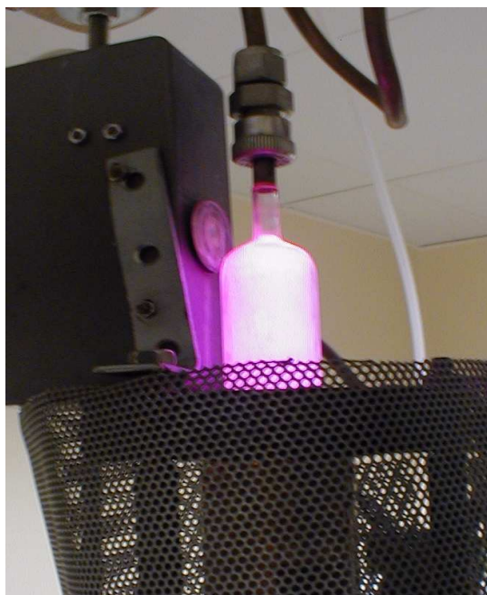
Figure 2.2 Photograph of the H-atom source.
