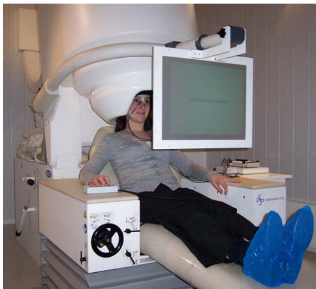
Figure 2.10 Participant in MEG system in magnetically shielded room Plastic overshoes are worn to prevent inadvertent introduction of ferromagnetic elements into the MSR.
