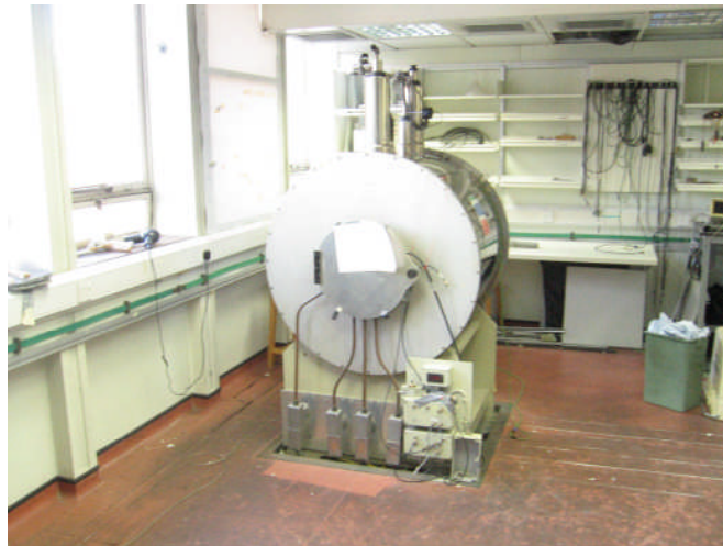
Figure 1.18 The Experimental MRI scanner used in the imaging studies described in this thesis. The scanner was installed on the fourth floor of the UCL Institute of Child Health in 1984.
