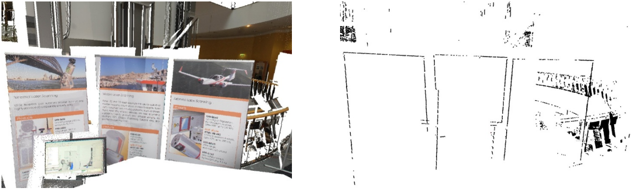
Fig. 8: A colored point cloud acquired with a V-Line terrestrial laser scanner from Riegl is shown on the left. The multi-pulse capability of the scanner facilitates 3D edge detection shown to the right, by selecting only first return pulses. LiDAR data is courtesy of RIEGL Laser Measurement Systems GmbH.
