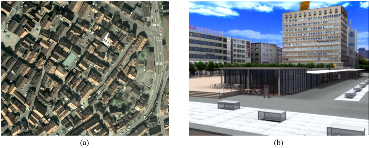
Fig. 1: (a) A DMC image as a typical representative for the bird's-eye view of aerial data acquisition. Image is courtesy of Intergraph. (b) The visualization from a pedestrian view of an architectural design combining existing urban data and planned data (Burkert, 2000).
