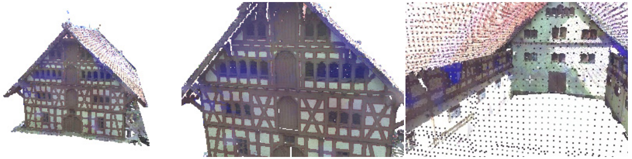
Fig. 4: A colored point cloud acquired with terrestrial LiDAR. While the point cloud gives a good impression of the object from a far away view point, when we zoom in the impression of a solid surface collapses.
