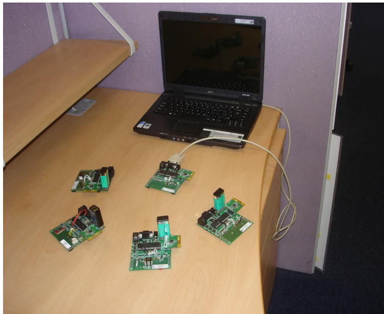
Figure 4.18: Experimental Hardware: the main setup components included a 9V power supply, Microchip PICDEMZ boards fitted with Chipcon CC2420 transceivers, ICD 2 debugger and a laptop computer
