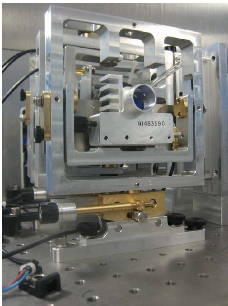
Figure 5.19 New mounts for the AODs with independent fine control of axial (Z axis) rotation about the centre of the crystal using the brass lead screw visible underneath the main frame. Rotation about the horizontal X axis uses the next half frame in whilst rotation about the Y axis to control the Bragg angle has a course manual setting about the clamped support mount just above the brass lead screw, and a fine lead screw control close to the crystal and not visible here 12 .
