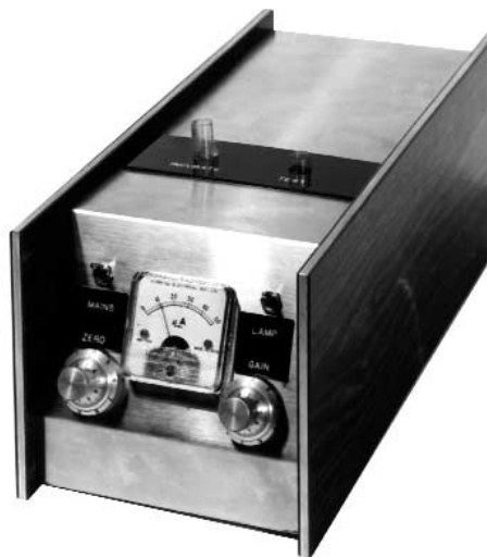
Figure 5: The first aggregometer made in the workshop at the Royal College of Surgeons in 1961. Born (1962b).
