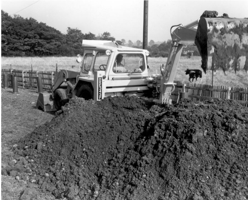
Figure 9: JCB backhoe loader, an example of the machinery used to prepare burial sites in 1967.
