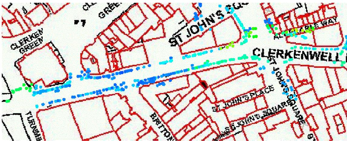
Figure 7: Clerkenwell Road 4 February 2005 at 15:05, GPS corrected to the pavement with detection of road crossings based on a change in track angle. This does not use any additional route knowledge.
