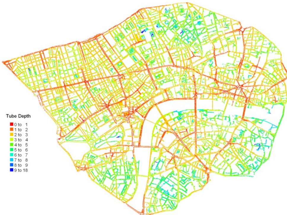
Figure 7: Tube Station Accessibility Analysis of Central London
