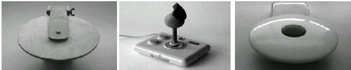
Figure 23: Version one of the Turntable. The turntable device utilised an analogy with the potter's wheel.
