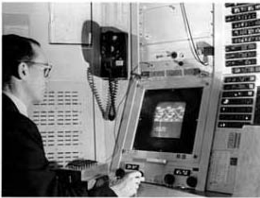
Figure 2: The display, a light pen, and a bank of switches were the interface on which Ivan based the first interactive computer graphics; he used the light pen to create engineering drawings directly on the CRT.
