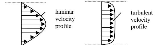
Fig. (C1): Velocity profile for laminar and turbulent flow (pipe, mechanically ventilated).
