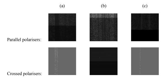
Figure 3: The cylindrical lenses (original (a), strip electrode (b) and electrode-on-top (c)) as seen through crossed and parallel polarisers, input polariser parallel to rubbing direction with 8V applied.
