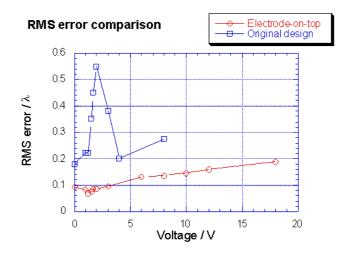
Figure 5: RMS error of original and new design of spherical microlenses
