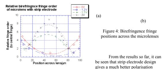
performance but there is still a disclination. The design with the electrode on top of the lens gives an improved polarisation performance and no disclinations.
