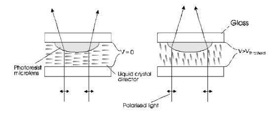
Figure 1: Basic design of liquid crystal immersed microlens
