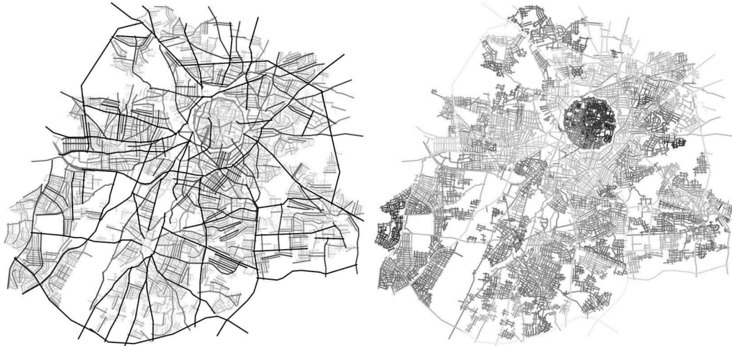
Figure 4: The continuity map of Nicosia, Cyprus, using an angle of 45°. The Figure has two types of visualisation (Figueiredo, 2004). In the left, the multilayer structure of the supergrid is highlighted. The darker lines roughly correspond to the 5% longest lines. In the right, “neighbourhoods” are highlighted by finding clusters of lines with similar line length. The intensities of grey are based on the average line length of the cluster. Note that the two parts of the Old Nicosia (centre) have slightly different intensities of grey. The map is a courtesy of the Space Syntax Laboratory (Konstantinos Kypris).
