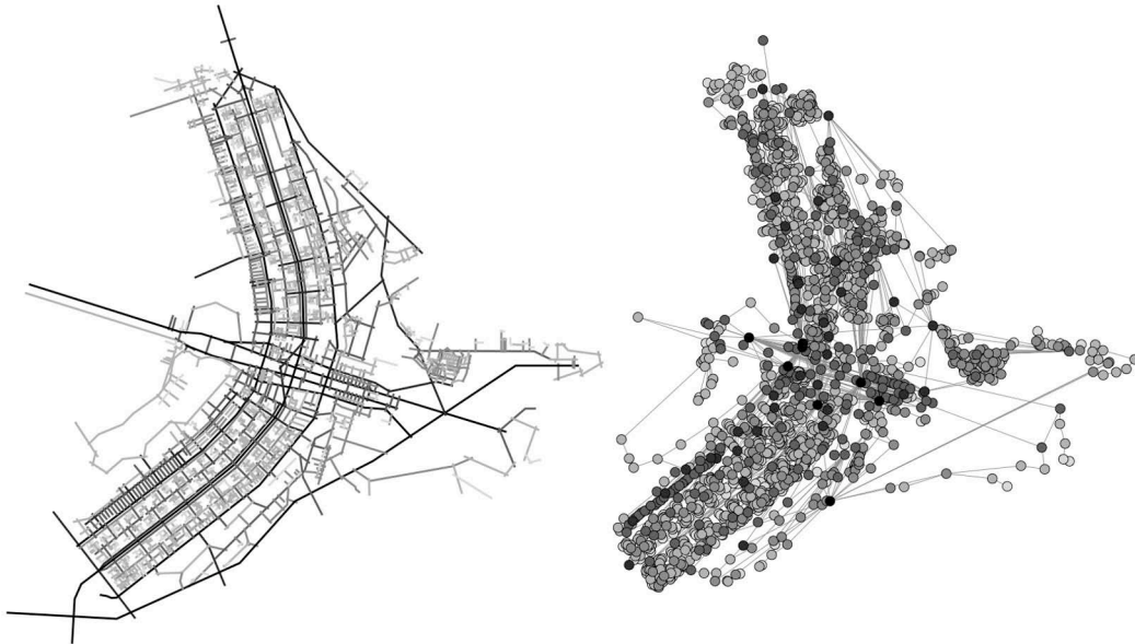
Figure 1: (Left) The continuity map of Brasília, Brazil (Holanda, 2002), using an angle of 45°. (Right) The underlying graph created by the continuity map (Figueiredo, 2004) where lines are nodes and intersections between lines are edges. The darker lines and nodes are the ones with high degree value. The degree or connectivity of a line is the number of lines that intersect that line. The degree defines the primary importance of a line in the system or, as cities are grids, the number of neighbours up to two steps.
