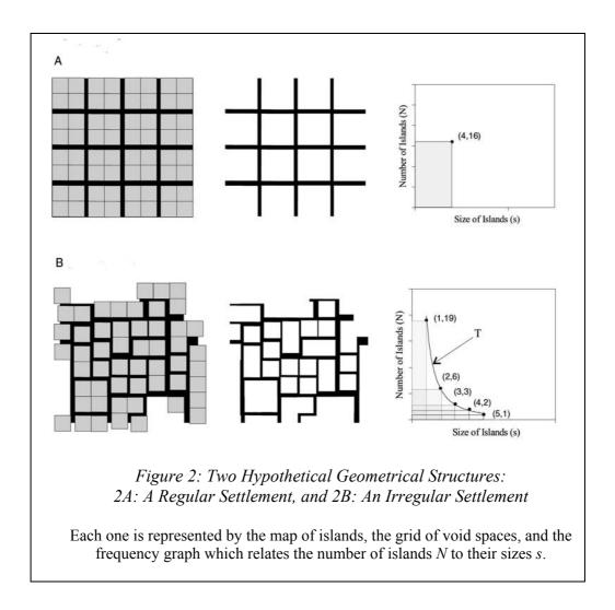
Figure 2A shows a regular grid, composed by a group of identical islands, distributed within a square area. It is really very simple to obtain global parameters from the local units of this regular structure. For example, as we observe, each island contains four cells
