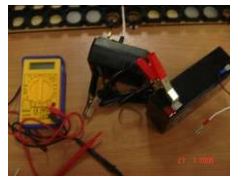
Multimeter, battery charger & battery
