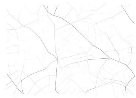
Figure 1.12a Choice analysis of part of north west London for trips of any length
