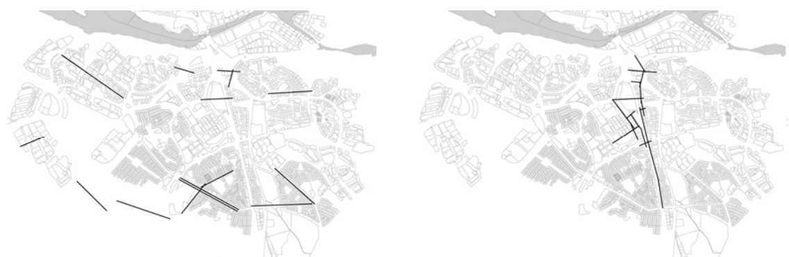
Figure 3.2. The most integrated lines in an area of the southern suburbs of Stockholm. Local integration to the left and global integration to the right.
