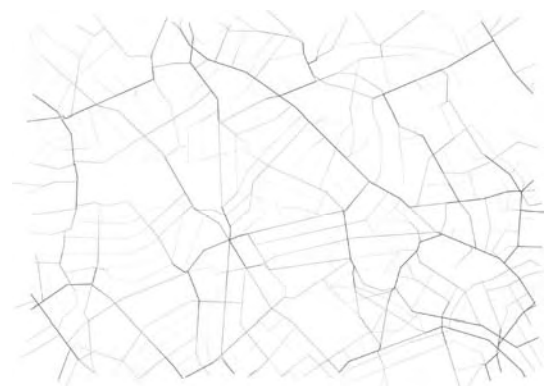
Figure 1.12b Choice analysis of part of north west London for trips up to 1.25km
