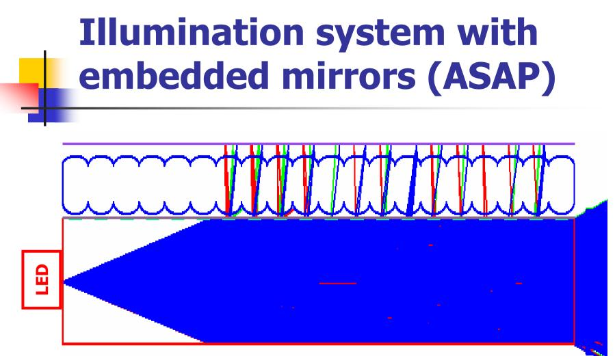
Mirror position,  $d: 10 \ \mu m$  to lightguide upper surface Mirror Width,  $w: 160 \ \mu m$
