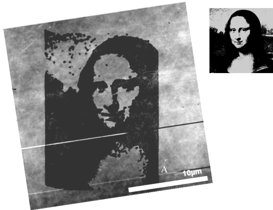
Figure 4.36: Sample ppvD67, possibly the smallest Mona Lisa in the world! Fabricated from PPV, the detail is missing due to overexposure and the fast shutter switching burned out the shutter controller at point A discouraging further attempts, but the smile is still there. Inset shows the monochrome bitmap used for the patterning.
