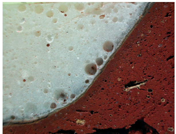
Fig. 7: Close-up of the reaction zone at the bottom of AT8, showing only a faint buff zone between the glass and the ceramic, and almost no discoloration.
