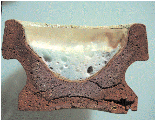
Fig. 4: AT2 with residual parting layer and buff and pink discoloration zones in the ceramic, consolidated with resin.
