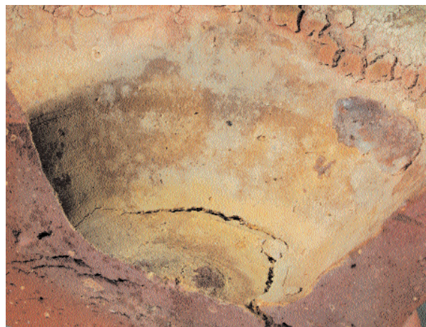
Fig. 24: Inside of AT1 after the firing and removal of the glass cake. Note the discoloration of the ceramic, and the patch of glass adhering to the ceramic (centre right).
