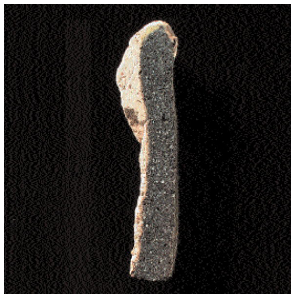
Fig. 1: GT 281 with an exceptionally thick coat of parting layer material near the rim.
