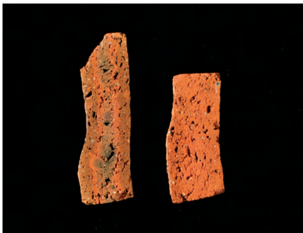
Fig. 20: Modern Nile silt ceramic, as received (left) and re-fired at 900 °C (right).
