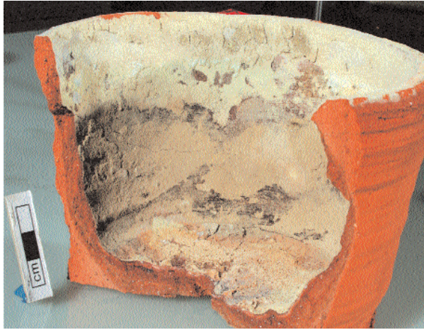
Fig. 8: A hand-made cylindrical vessel after firing a salt-containing batch to produce semi-finished glass. The vessel was deliberately broken to reveal the discoloration of the ceramic.
