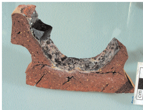
Fig. 13: The glass separated badly from AT4, with some glass still attached to the ceramic.
