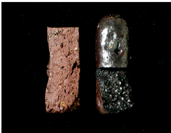
Fig. 23: Modern Nile silt ceramic, re-fired at 1150 °C (right) and 1200 °C (right).
