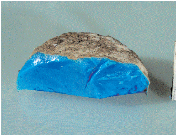
Fig. 18: The ingot from AT3, with residual parting layer material attached.
