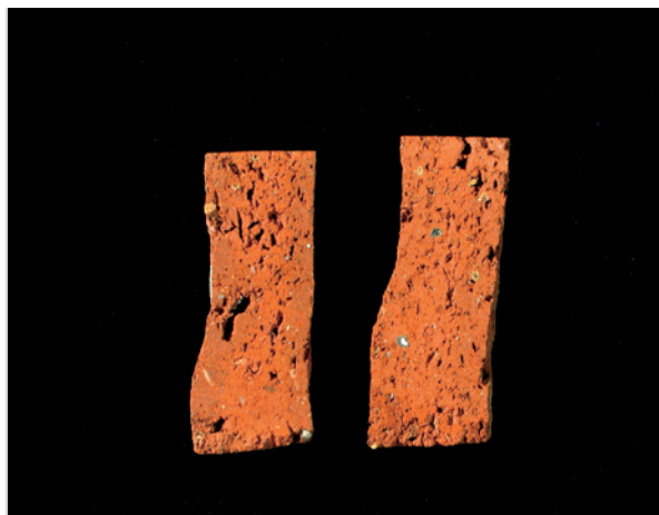
Fig. 21: Modern Nile silt ceramic, re-fired at 950 °C (right) and 1000 °C (right).
