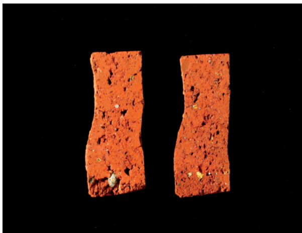
Fig. 22: Modern Nile silt ceramic, re-fired at 1050 °C (right) and 1100 °C (right).
