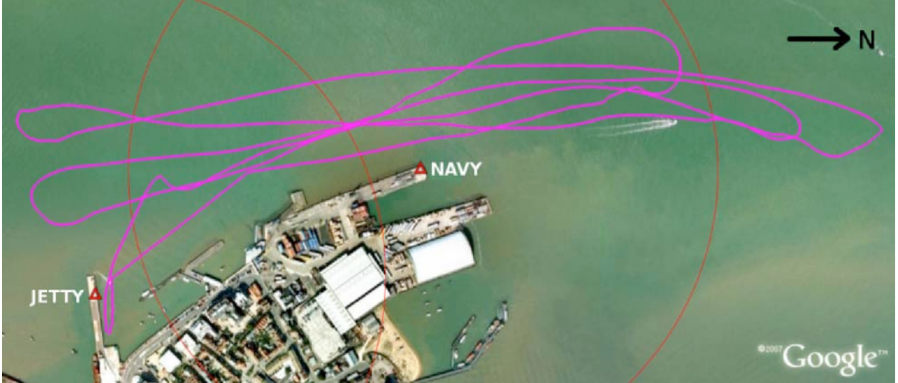
Figure 4: Plot of THV Alert 's course, showing total station locations with 400 m range circles
