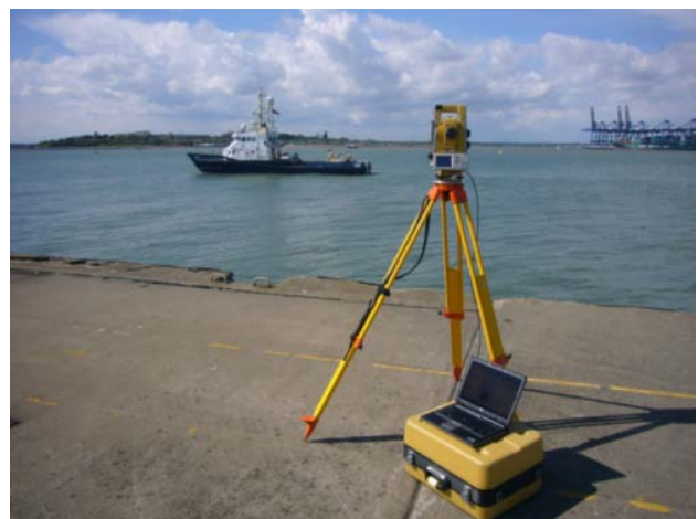
Figure 2: Total station tracking THV Alert
