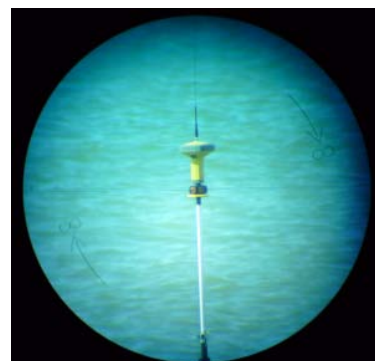
Figure 3: GPS receiver and prism on THV Alert , viewed through the total station telescope
