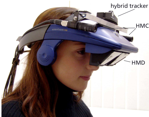
Figure 2: ARTHUR See-through head mounted display (HMD).
