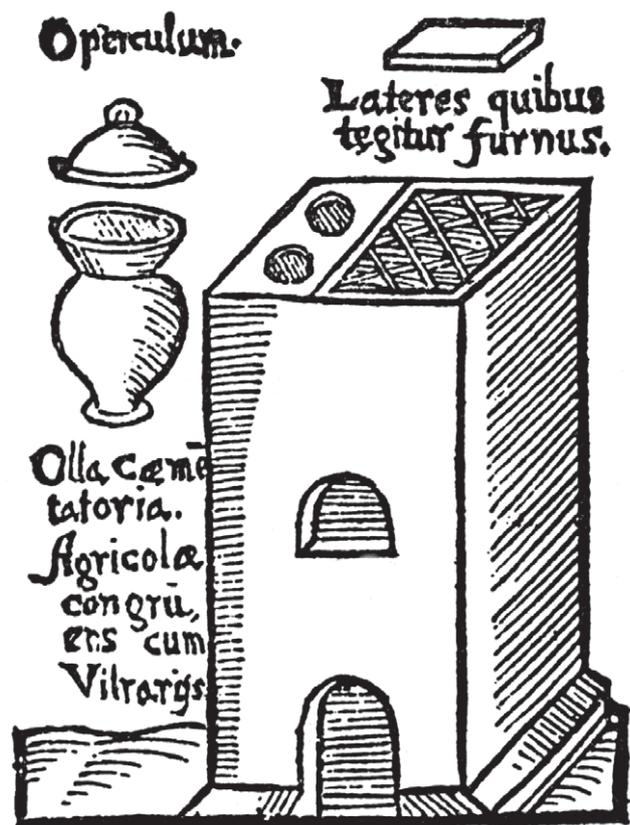
Figure 14: Reinterpretation of Fig 13 by Libavius in which the crucible lid appears perforated as Agricola advised, although Fig 13 does not show this detail. (Illustration from Rex 1964, 74).
