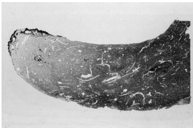
Figure 1: Cross section through a crucible fragment from Stäfa-Uerikon. Note the very limited vitrification layer near the rim of the vessel, top left. Width of image ca. 3 cm.
