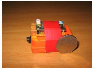
Figure 1 – A battery-powered MTx sensor connected to a connectBlue WiFi module via RS232
