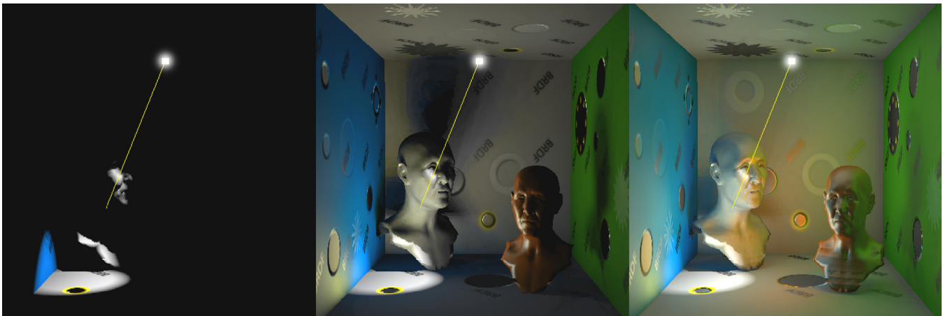
Figure 16: Direct light (left, 100 fps), one indirect bounce (middle, 7.4 fps) and two indirect bounces (right, 1.4 fps).
