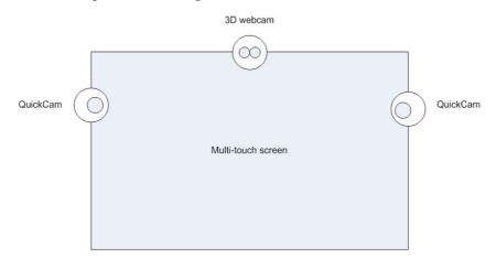
Figure 4: The multiple camera arrangement
