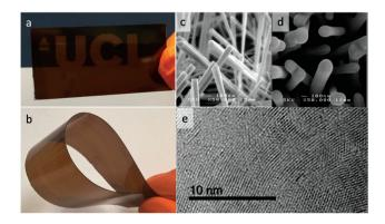
Fig. 1 (a) GCN film deposited on glass. (b) GCN film deposited on acetate plastic. (c) SEM image of uncoated WO<sub>3</sub> nanorods. (d) SEM image of WO<sub>3</sub> nanorods coated with GCN (e) TEM image of GCN film coated directly onto a holey carbon grid, showing lattice fringes.
