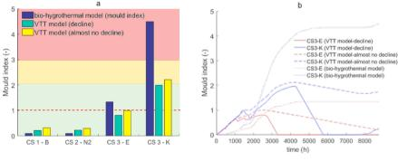
Fig. 2. Mould index (a) according to bio-hygrothermal and VTT models. Comparison of mould index as function of time for CS3-K (b).
