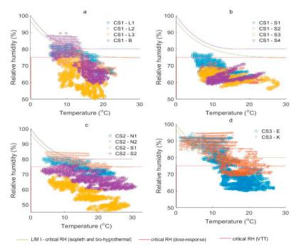
Fig. 1. Hourly data points against the critical relative humidity curves defined for each model, case study 1 (a, b), 2 (c) and 3 (d)
