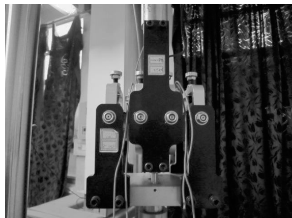
Figure 1. A newly-developed mini-4PB test apparatus on the MTS for CAMs
