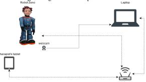
Fig. 2. Diagram of the setup connections.
