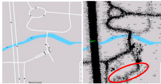
Figure 1. Detection of a missing road on the map using the trajectories of users.
