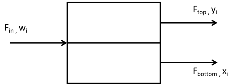
Figure 4 - 9: Liquid-liquid equilibrium stage used to derive Rachford-Rice objective function
