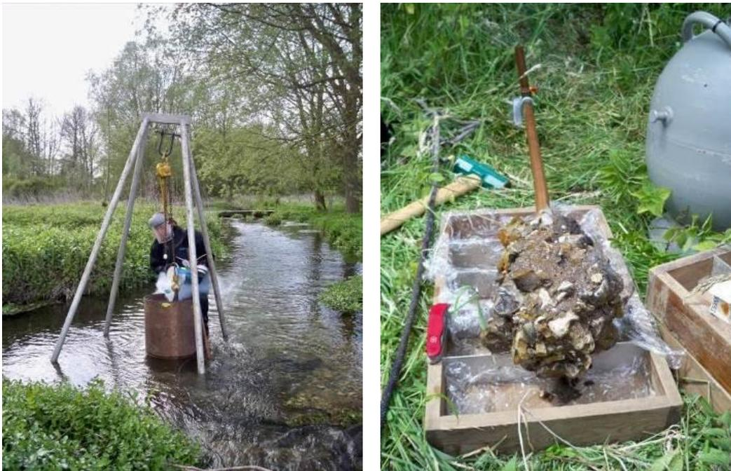
**Figure 2.9** Photographs of freeze core sampling (left, site 8) and thawing core (right)
