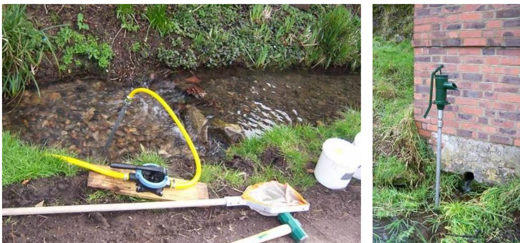
**Figure 2.7** Modified (left) and unmodified (right) Bou-Rouch pumps for hyporheic sampling.
