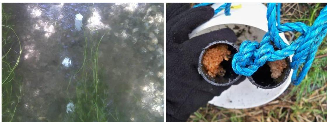
**Figure 2.8** Vacuum-pumping pipes (left) and artificial substrates contaminated by *Salmo trutta* roe (right), both from site 10.
