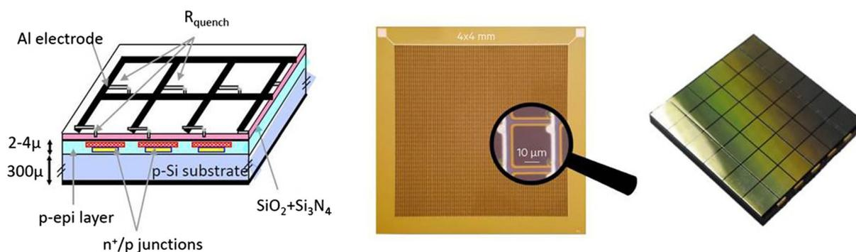
**Fig. 3** SiPM principle: SiPM tiles contain several thousand single-photon APDs operating in Geiger mode, with an output signal for the tile that is proportional to the total number of detected light photons.
