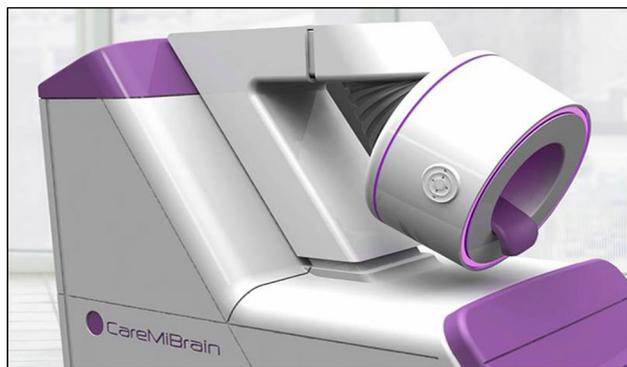
**Fig. 8** Dedicated brain PET: novel designs for dedicated brain PET are appearing on the market with compact systems such as the illustrated system from OncoVision which has better than 2 mm spatial resolution
