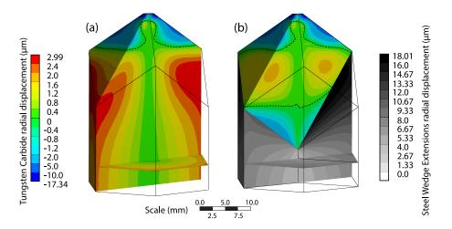
FIG. 3. Radial deformation in (a) hexagonal anvil and (b) replacement cubic anvil and deformation wedge extensions, from finite element analysis. The red-blue colour scale applies to tungsten carbide parts and the grey scale applies to steel components. The dashed line is zero radial displacement iso-surface in the tungsten carbide components. For details of the models, see the text.
