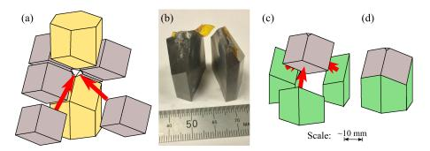
FIG. 1. Deformation anvils in the DT-Cup. (a) Arrangement of the 6 cubic and 2 hexagonal anvils in the DT-Cup, (b) example of broken anvil, and [(c) and (d)] replacement "deformation wedge extensions" with cubic anvil.
