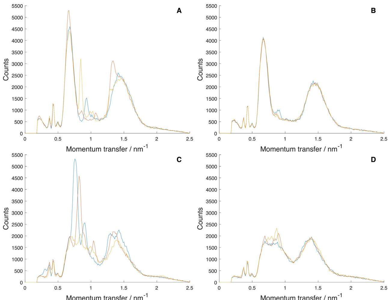
**Fig. 4.** Plots (A) and (C) show the profiles in triplicate of samples 2 and 11, respectively, when translational stages were not used. Plots (B) and (D) are the corresponding profiles when intra-screening translational stages were introduced – preferred orientation effects caused by paracetamol were greatly reduced.
