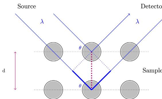
**Fig. 1.** X-ray incident on two parallel planes at an angle  $\theta$ , with photon wavelength  $\lambda$  and planar spacing  $d$ . The thicker ray line represents the additional path length traversed in a reflection from the lower plane which, for a coherent scattering event, is an integer multiple of the X-ray wavelength, satisfying Bragg's law.
