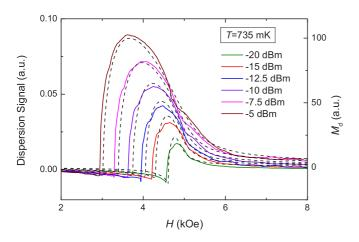
FIG. 5. Dispersion signals measured in MnCO<sub>3</sub> at T = 735 mK and at several values of input rf power (shown in the figure) during a down-field sweep. Dashed lines represent values of  $M_d$  calculated as described in Sec. III C.
