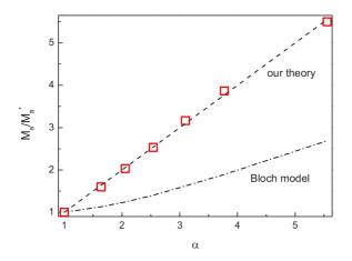
FIG. 7. Normalized values of the absorption signal at the critical field  $H = H_{c1}$  as a function of quantity  $\alpha(H_{c1}, \sqrt{P/P^*})$  defined by Eq. (45) obtained from the experimental data presented in Figs. 4 and 6 (open squares). The lines are the corresponding dependences predicted by our theory (dashed line) and by the conventional Bloch approach (dashed-dotted line).
