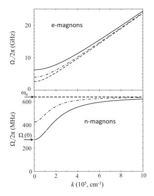
FIG. 1. The spectra of *e*-magnons and *n*-magnons in  $MnCO_3$  in the static magnetic field of 0.2 kOe and at two values of temperature of 5 K (dashed-point line) and 1.4 K (solid line). The dashed lines show corresponding spectra in the case when coupling between electron and nuclear oscillations is neglected.
