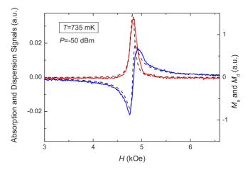
FIG. 3. Absorption (solid line, red) and dispersion (solid line, blue) signals measured in MnCO<sub>3</sub> at T = 735 mK and at a low input rf power of P = -50 dBm. Dashed lines are the ac magnetization components  $M_a$  and  $M_d$  calculated as described in Sec. III C.
