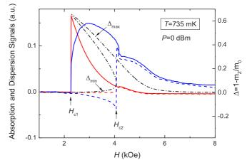
FIG. 6. Absorption and dispersion signals measured at T = 735 mK at the highest input rf power of P = 0 dBm during up-field (dashed lines) and down-field (solid lines) sweeps. The dashed-dotted line is the result of numerical calculations for  $\Delta = 1 - m_Z/m_0$  as described in Sec. III C.
