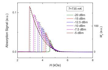
FIG. 4. Absorption signals (solid lines) measured in MnCO<sub>3</sub> at T = 735 mK and at several values of input rf power (shown in the figure) during a down-field sweep. Dashed lines represent values of  $M_a$  calculated as described in Sec. IIIC.
