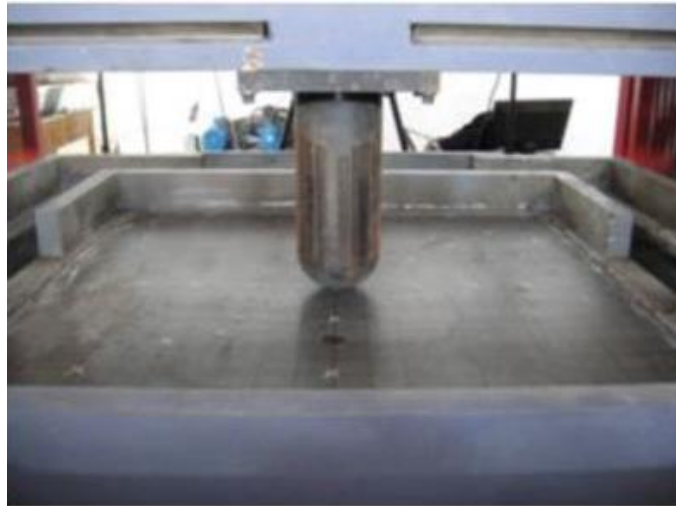
Figure 15. The dropped test on a rectangular plate impacted by a rigid indenter (Liu et al. 2016).
