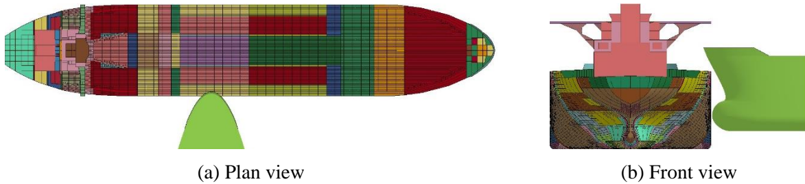
Figure 4. Collision angle and location considered in the present parametric studies.
